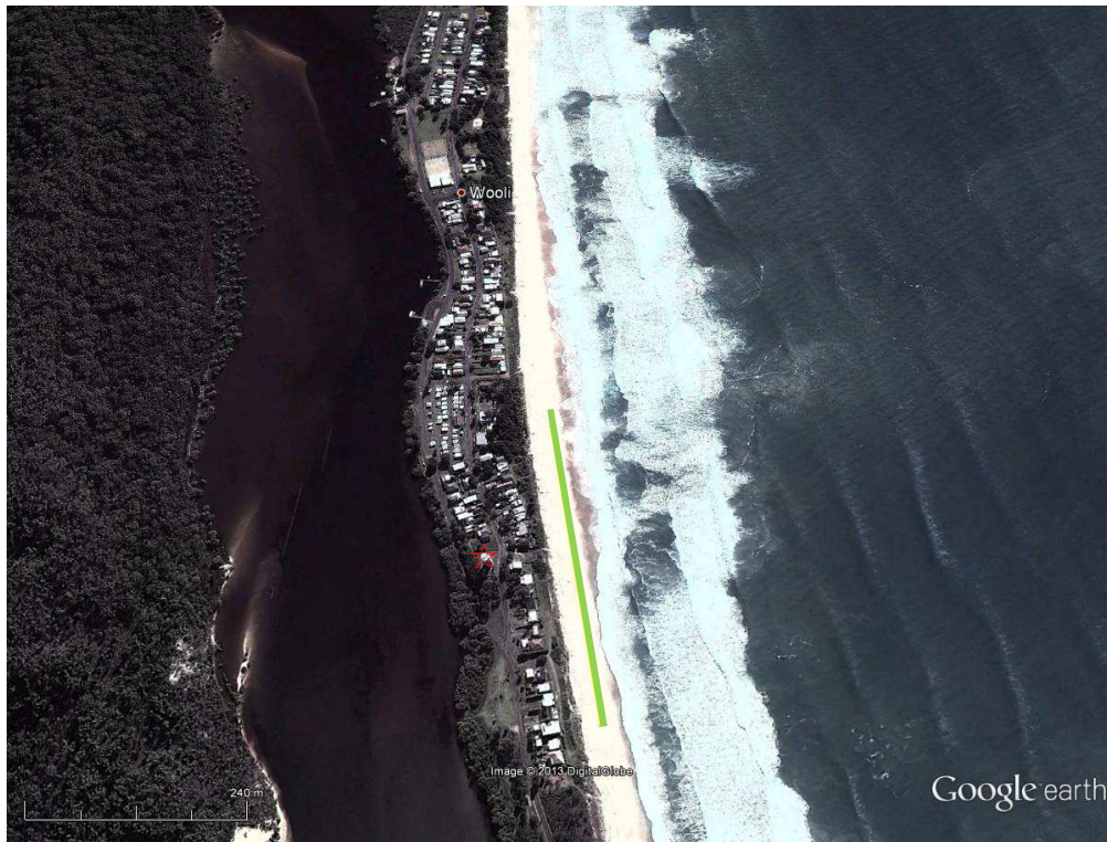
Figure 1.1. The useable 1 field of view from the coast-cam system is represented by the green line, with the Wooli water tower denoted with the star, which is 33.5 m above Australian Height Datum (AHD), which is approximately mean sea level (MSL).
